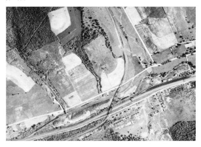
As part of the changes to the PRR and Montour tracks going into McDonald Mine, the Carnegie Coal Company allowed the PRR to install a track that went beneath the McDonald Viaduct to connect with the Panhandle's JO Yard, which paralleled the main track. The aerial photograph from 1939 shows the track arrangement for
