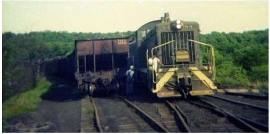
Loaded hoppers have been pushed up the hill from Mine #10 onto the siding. The train crew is now using a cross-over switch to run around the cars and couple onto the front of the train.
