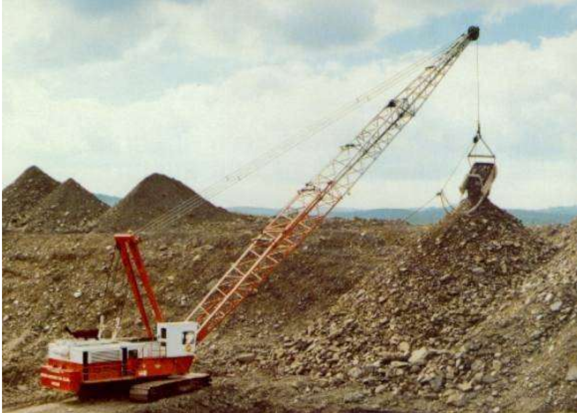
A dragline is moving dirt and rock overburden at a strip mine.
