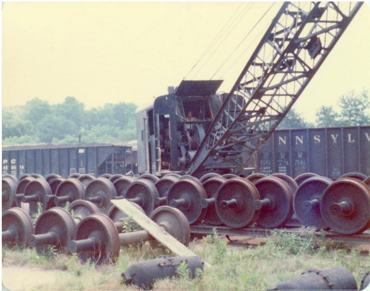
The X1 crane unloads wheel sets at the Car Shop. Charles A. Ross photo
