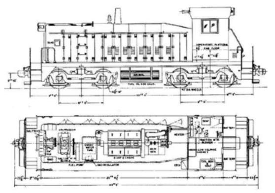
Schematic diagram of an SW-9 Locomotive
