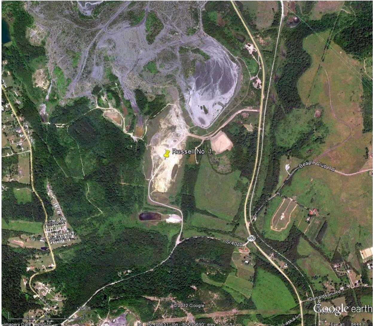
The topographic map shows the tipple and extent of the mining operation. The pipeline and small pond provide a reference to the tipple site mentioned above.
