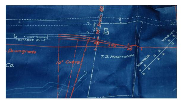
The new connection passes beneath the south end of the tipple, crosses over the original runaround track and connects to the lump coal loading track. Note that the tipple can load three grades of coal, lump, nut and slack (see the article of the Champion coal washer for more information). There is also a supply track and a 36-inch concrete pipe that drains the mine water into Robinson Run.
