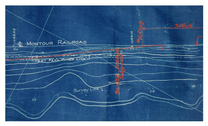
As we continue timetable eastward down the new connection we see the gradient increase from 1.7% to 2% as the right-of-way no longer parallels the hillside but begins to cut across the elevation lines as it descends from 1,025 feet to below 1,000 feet.
