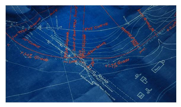
The new track passes beneath the McDonald Viaduct and connection with the tracks in the loaded yard for the McDonald Mine tipple. There is also a runaround track and all switches are No. 8 frogs rated for 5 to 10 mph.
