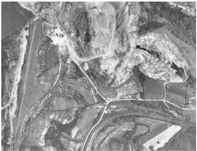
This is an enlargement of the 1958 photo that shows the Russell No. 2 tipple. Trucks from the strip pits would back into a dump to the right of the road and coal was conveyed underneath the road to the tipple.
