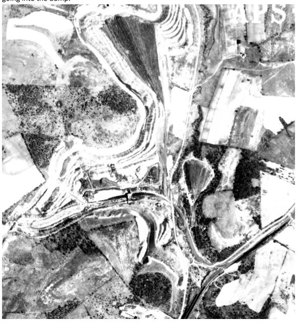
This 1958 photo clearly shows a string of hopper cars on the spur leading to Russell No. 2 and active strip mining in progress. The Montour is using the old track to the former Champion waste dump to reach the mine tipple at the top of the photo. By this time, Champion was dumping its waste in the valley west of PA Route 980 across from the coal washer.
