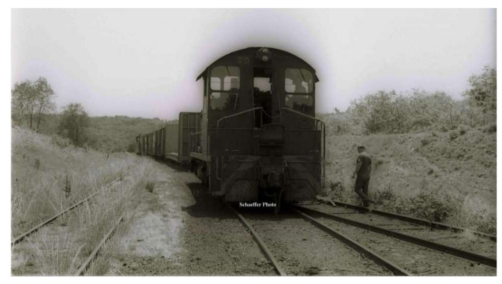
After shoving its cars all the way from Bethel Park, engine 75 backs down the east leg of the wye. It will run along each leg of the wye, recouple to its train and then proceed west with the engine leading the train. The storage siding track can be seen to the left of the train.
